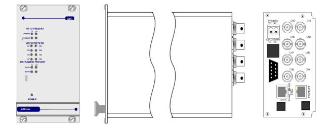
The **AMG3784ERN** is a rackmount eight channel video receive unit designed to receive 8 video signals from a singlemode optical fibre ring. It also provides one bi-directional data channel via a low speed data interface, plus full duplex 100BaseT Ethernet connectivity around the ring.
